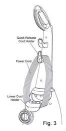
4. Turn the quick release cord holder to the left or to the right to unwrap the power cord. (Fig. 4)
